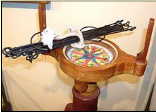
CIRCUMFERENTOR (Surveyor's Compass) With Gunter's Chain Wikipedia Website
